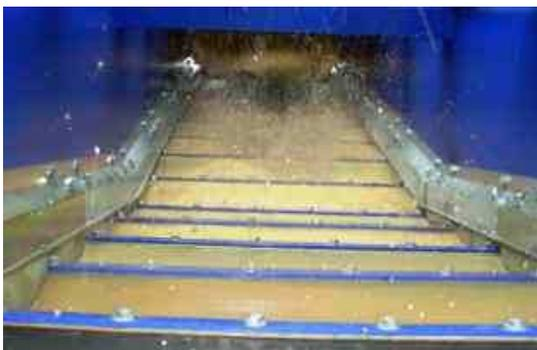
**Siebmatte in Action (Spannwellensieb)**
